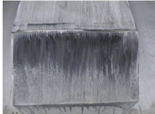
Figure 5. Oil / soot streak flow visualization of the Ahmed body rear for a 35^\circ slant angle.
