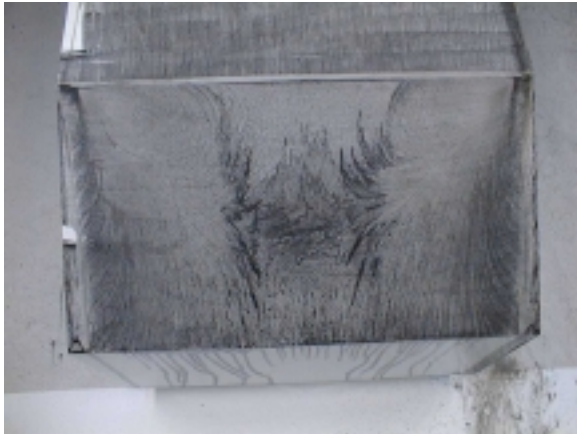
Figure 4. Oil / soot streak flow visualization of the Ahmed body rear for a 25^\circ slant angle.
