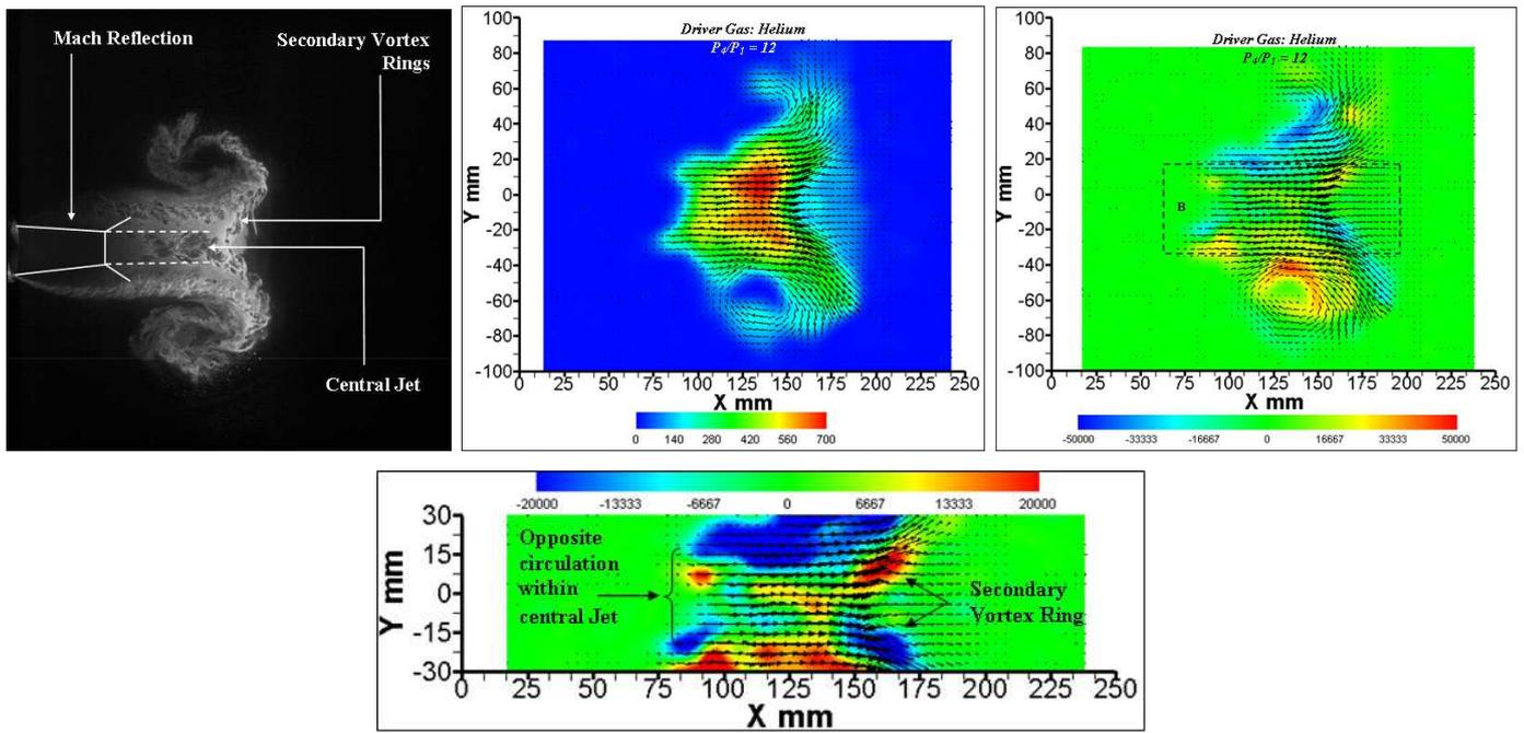
Figure 2: 30mm straight nozzle,  $P_4/P_1 = 12$  at vortex ring structure (left), velocity magnitude (centre), vorticity (right), and shear layer with secondary vortex rings (bottom)
