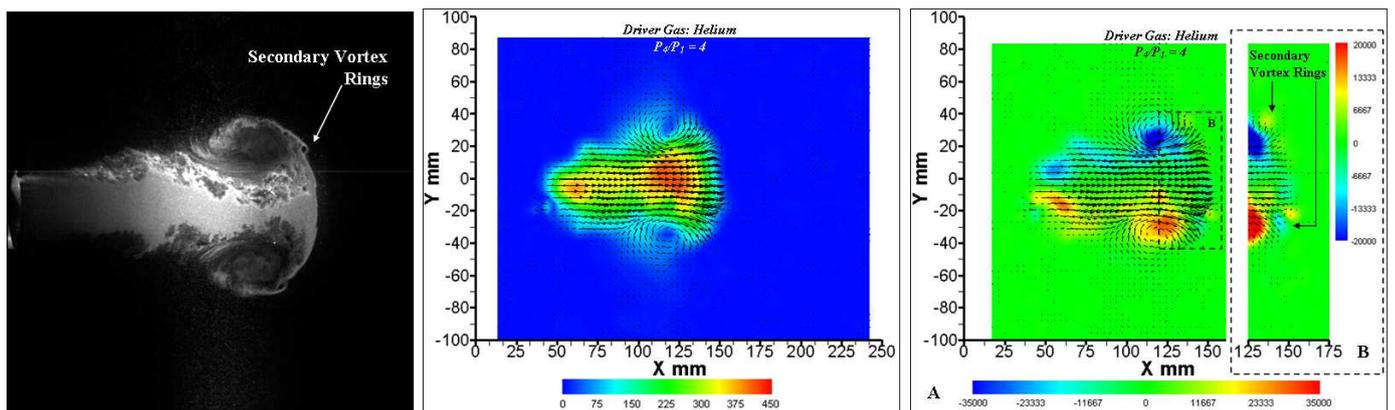
Figure 1: 30mm straight nozzle,  $P_4/P_1 = 4$  at vortex ring structure (left), velocity magnitude (centre), and vorticity (right)
