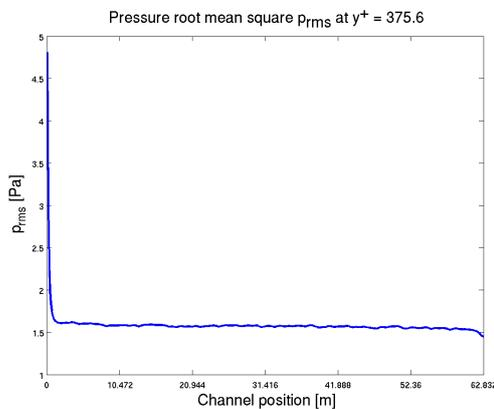
Figure 3: Pressure fluctuations after mass flow rescaling
