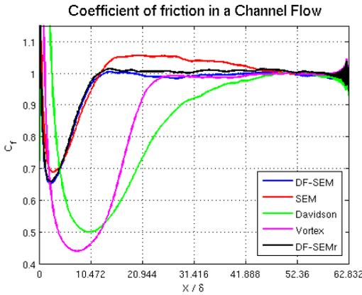
Figure 1:  $C_f$  performed in Channel Flows,  $Re_\tau = 395$ , using different inlet methods
