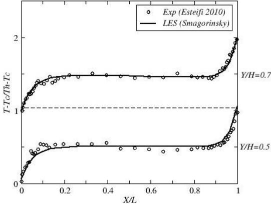
Figure 1: Time-averaged temperature profiles at two different heights inside the cavity (inclination of the cavity  $15^\circ$ )
