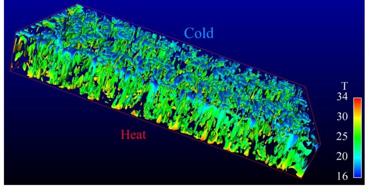
Figure 2: Iso- $Q$  contours coloured by the temperature (inclination of the cavity  $15^\circ$ )
