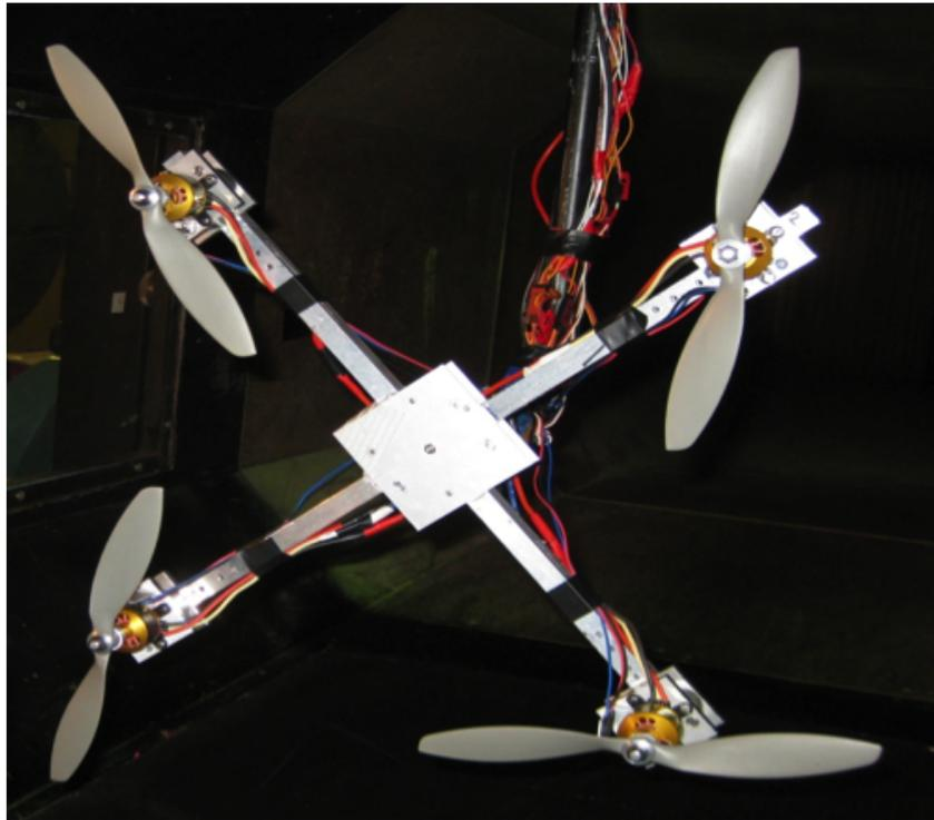
Figure 1: Quadrotor test-rig with adjustable rotor spacing, flight orientation and force balance position
