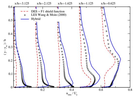
Figure 9.  $u_{rms}$  profiles over the aerofoil
