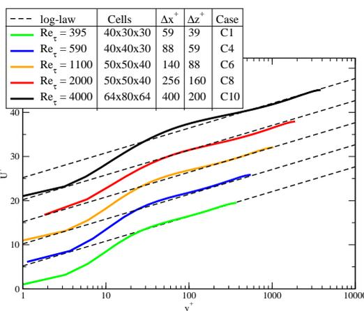
Figure 4. Velocity profiles at different Reynolds numbers.
