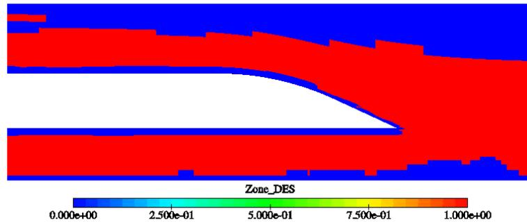
Figure 15. LES and RANS zones on DES simulation
