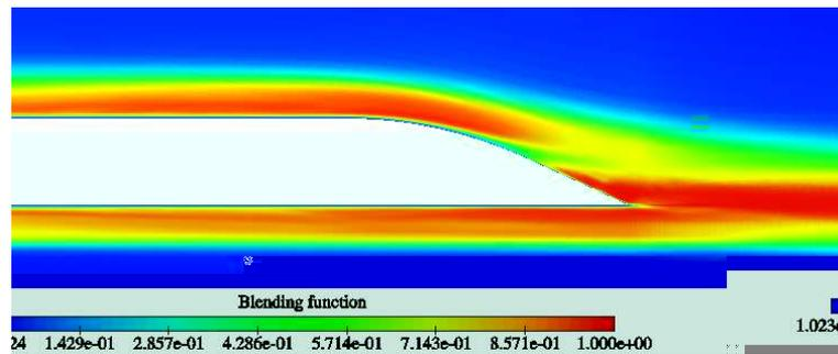
Figure 14. Blending function contours for the hybrid model
