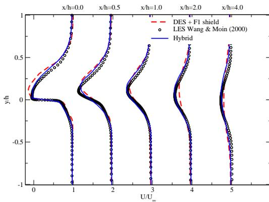
Figure 12. Velocity profiles at the wake
