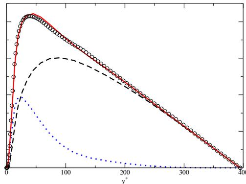
Figure 2. Shear stress at  $Re_\tau = 395$
