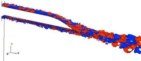
Figure 10. Iso-contours of  $u'$ , hybrid model
