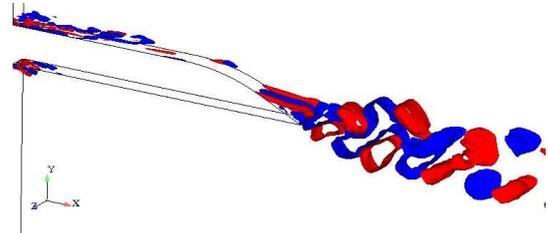
Figure 11. Iso-contours of  $u'$ , DES model
