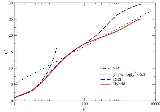
Figure 5. Velocity profiles at  $Re_\tau = 4000$
