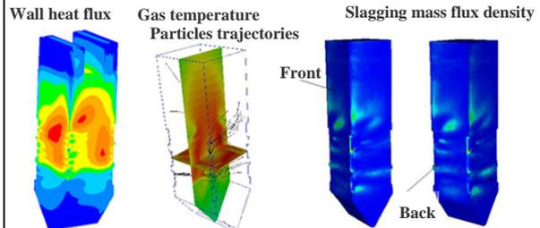
In the hopper and burners region, "slagging" is investigated with *Code\_Saturne*® using an homogeneous Eulerian model to compute the temperature and flowfield of the carrying phase and a high accuracy Lagrangian approach to track pulverized coal particles individually (wall-interaction modelling takes into account the surface condition, particle physical properties, velocity and angle of incidence).
