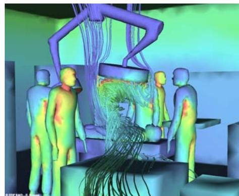
*Code\_Saturne*® enables an accurate representation of the equipment, medical staff, patient and HVAC (heating, ventilation and air conditioning) in order to determine zones where contamination risks are high and to evaluate the efficiency of the ceiling ventilation device.
