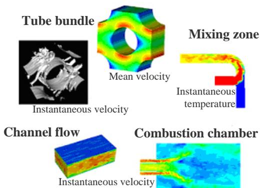
Large Eddy Simulation (LES) enables a refined description of local and instantaneous variables in turbulent flows (spectral analysis, local extremes) with immediate application to acoustics, structural analysis and thermal structure loading.
