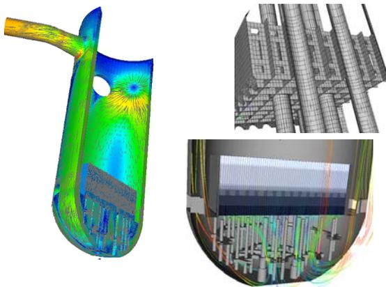
In 900 and 1300 MW Pressure Water Reactors, knowledge of flow conditions in the lower core is especially important to study **deformation and fretting of the fuel assemblies**.
