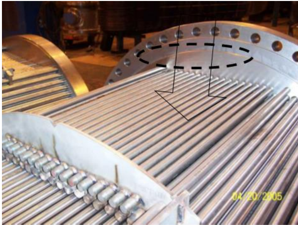
Figure 6: Typical layout of impingement rods in a heat exchanger bundle. (INEOS internal image file [1])
