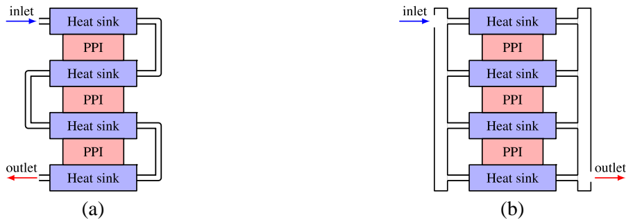
Fig. 9. Water-cooled PP stack configurations: (a) series and (b) parallel
