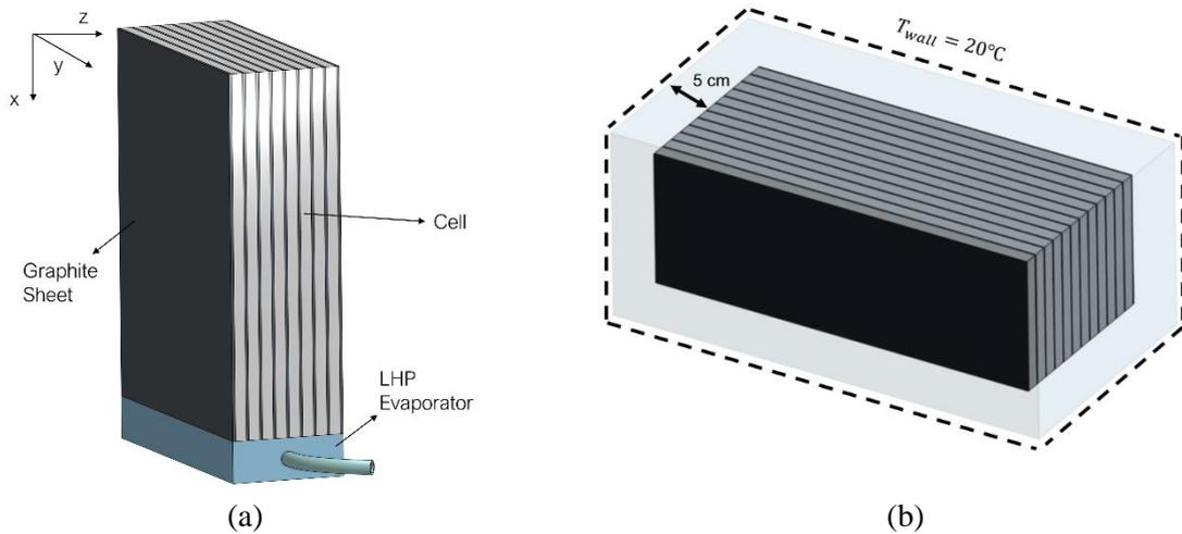
**Figure 1:** Schematic of (a) the proposed BTMS design [5] and (b) of control volume used in the free convection numerical simulations.
