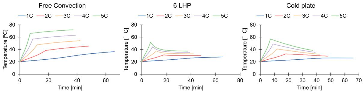
**Figure 3:** Comparison between the three considered BTMS over the 5 different driving cycles; charging times are 36 minutes for 1C, 18 minutes for 2C, 12 minutes for 3C, 9 minutes for 4C and 7 minutes for 5C.
