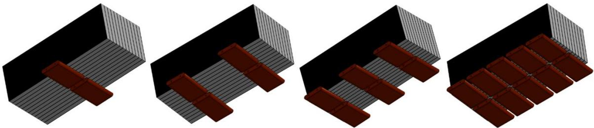
Figure 2: LHP based BTMS with varying number of 2,4,6,10 LHP evaporators.
