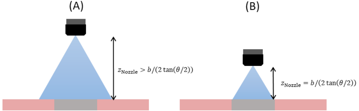
Figure 2: Depiction of the relation between the impact area of the spray and the ME surface area at varying nozzle-to-surface distances.
