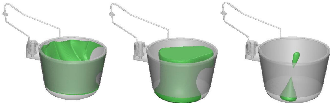
Figure 4a-c: Iso-surface of liquid fraction showing the solidification front at t=5000s , 30\,000s and 57\,000s .
