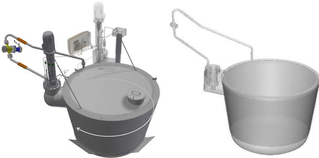
Figure 1: a) Discharge HTF loop overview b) CFD model including storage material, steel vessel, discharge HTF jacket, pump and simplified heat exchanger.
