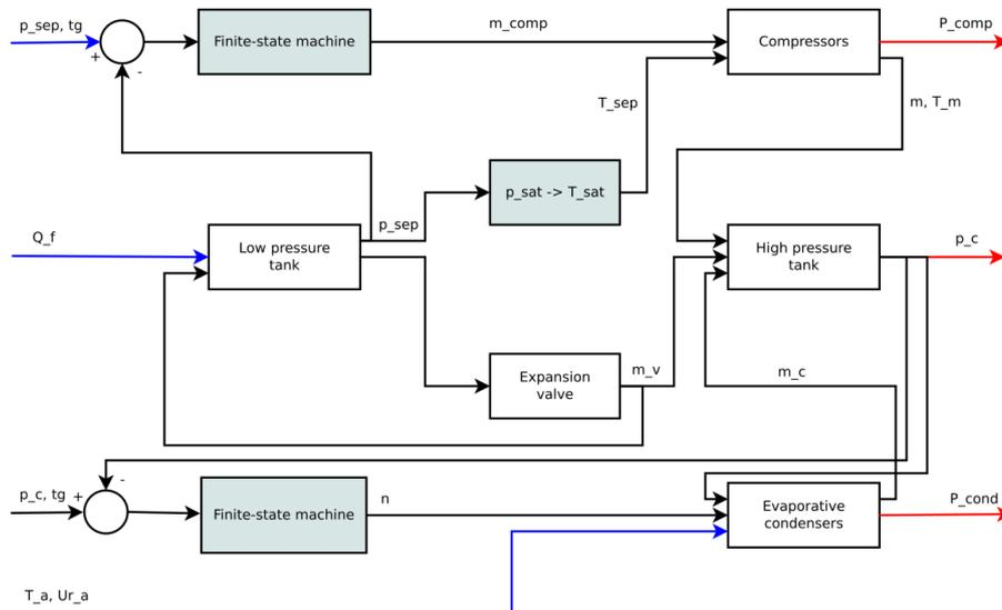
**Figure 1:** Full primary refrigeration loop model block diagram.
