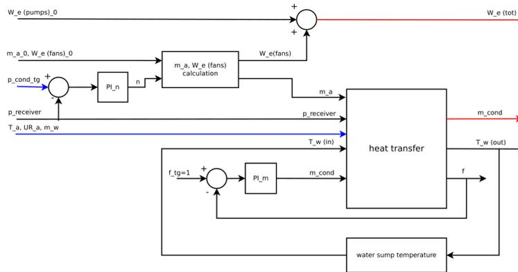
**Figure 2:** Evaporative condensers function block.
