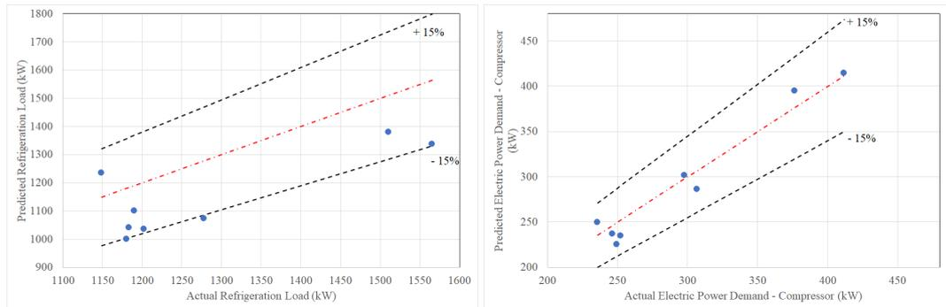
**Figure 3:** Power demand for the compressors (left) and refrigeration load (right): actual and predicted values.
