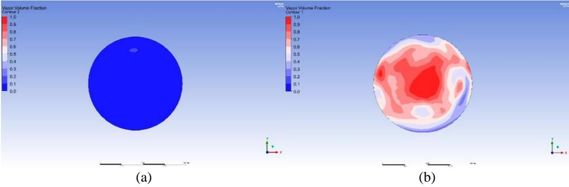
**Figure 5:** Void fractions in WMS position at 2 m/s (a) and 1 m/s (b) inlet flow.
