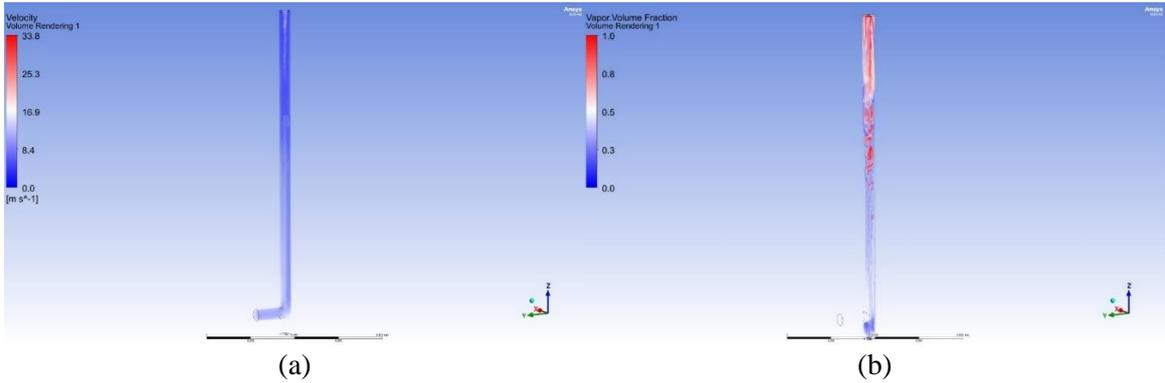
**Figure 4:** Local velocity (a) and void fractions (b) at 1 m/s inlet flow
