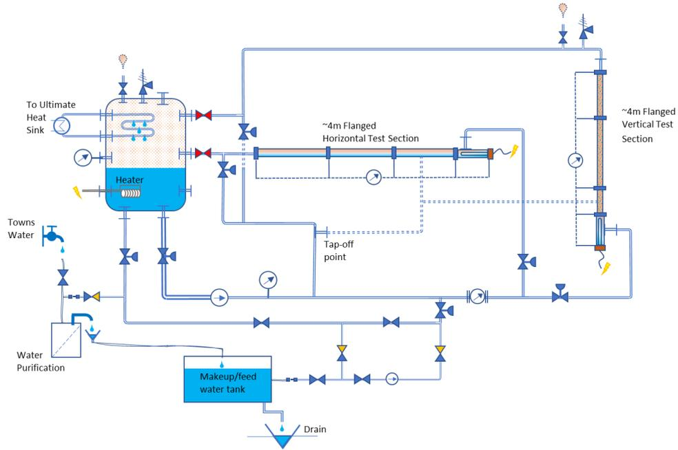
**Figure 1:** The Thermal-Hydraulics Open-access Research (THOR) facility: high-level P&ID.
