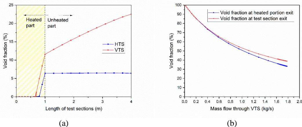
**Figure 2:** Steam generation capability in THOR's test horizontal and vertical test sections: (a) shows void fraction evolution over the length of each section, and (b) void fraction dependency vs mass flow in the vertical test section
