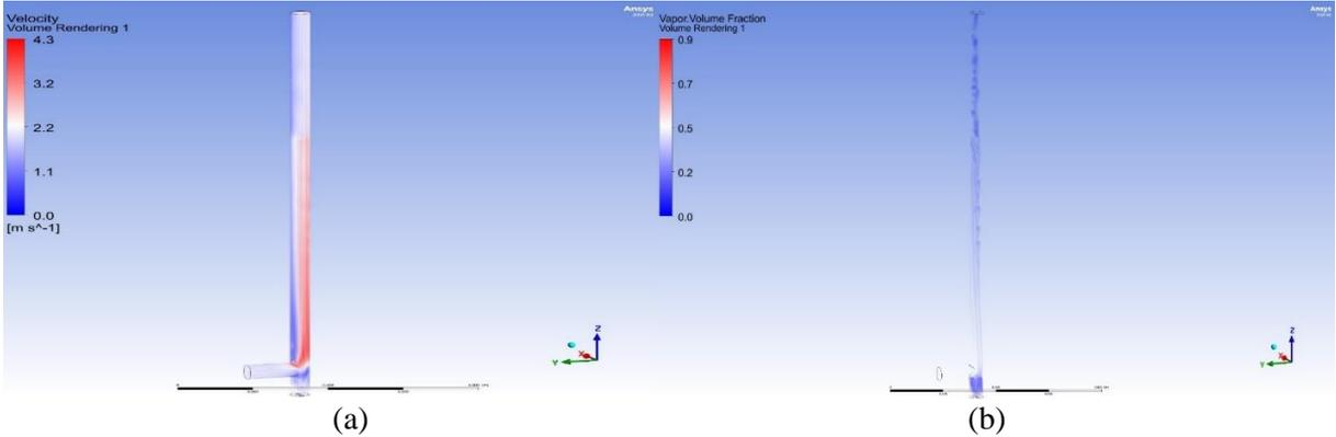
**Figure 3:** Local velocity (a) and void fractions (b) at 2 m/s inlet flow
